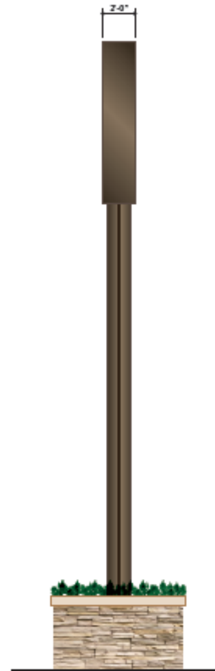
2 Monument Pylon - Side View SCALE: 3/16"=1'-0"
